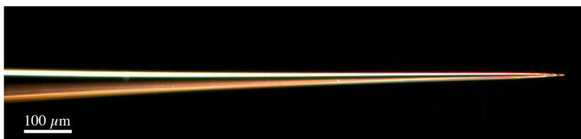
The quality of the needles is critical for high through-put. Needles should be pulled on any horizontal puller of the Sutter brand series using 1.0 mm OD borosilicate capillaries with omega dot fiber (e.g. Frederick Haer & Co, # 30-30-0). The settings will be different for
