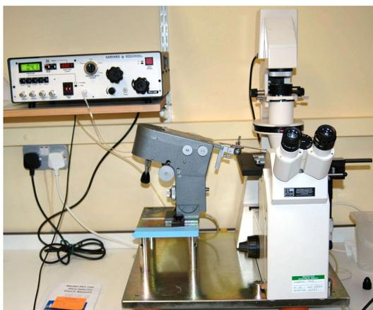
The injection set-up consists of two parts: an inverted microscope equipped with a 20x lens and a micromanipulator, and an air-pressure injecting device (e.g., Narishige IM-300 Microinjector) connected to the needle holder. Bright field or Nomarski diascopy are most appropriate to monitor injections. The micromanipulator can be attached to the stage or not, but if it is not, it should be firmly attached to the bench.
